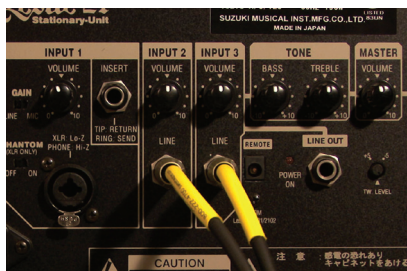
1/4 INCH CABLES PLUGGED INTO 2121 REAR
