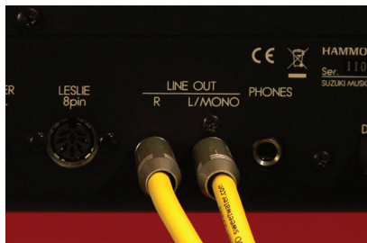
1/4 INCH CABLES IN JACKS ON BACK
