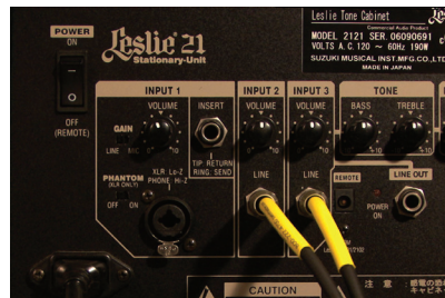
1/4" CABLES PLUGGED IN 2121 REAR
