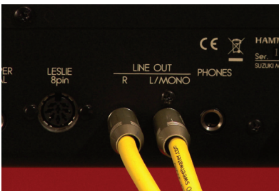
1/4" CABLES IN JACKS ON BACK OF SK
